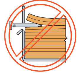
Nail at Wrong Angle
